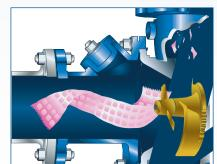
Solids reduction and blending Prior to entering the casing, large solids are chopped and reduced in size to ensure passage through optional disintegrator blade can be added at the inlet to break up large turbulence, thereby reducing power solids and facilitate entry into the consumption and improving NPSH. suction for further cutting by the impeller
